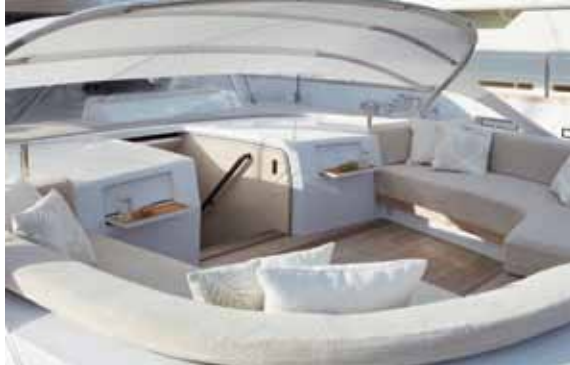
Left: the sunken aft cockpit replaces the need for deckchairs on the aft deck which would roll around when Twizzle is heeled over, and above, the main cockpit
